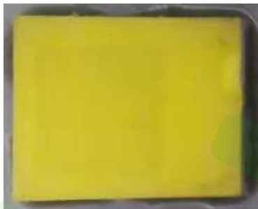
Conventional 2016LED, epoxy molding
